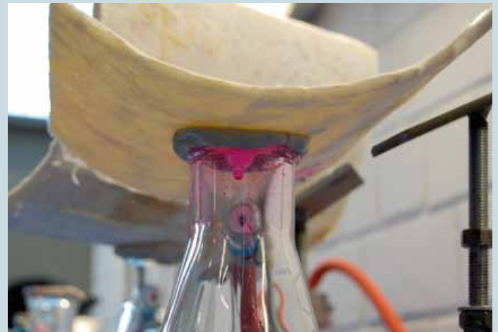
Tightness testing: liner not tight
