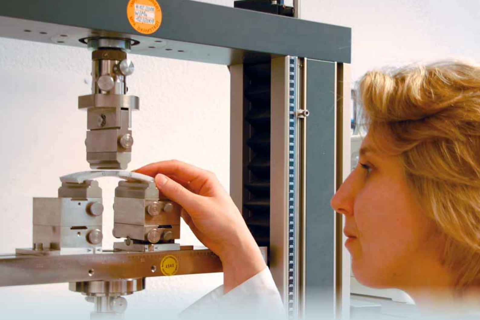
Test engineer Tatjana Kijan preparing a three-point bending test
